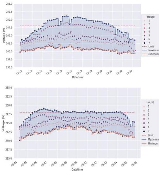
Figure 3 Voltage levels in the network without and with control respectively
